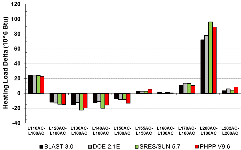
Figure B20-3. HERS BESTEST Tier-1 Example Results – Delta Annual or Seasonal Heating Load (L110AC - L202AC), Colorado Springs, CO
